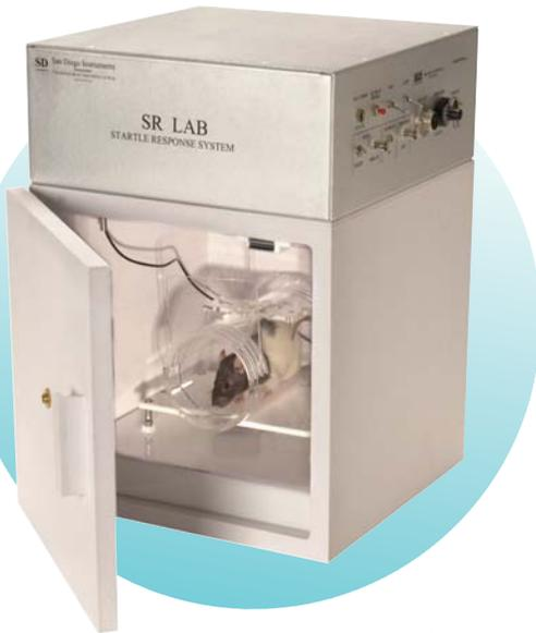
*Complete SR-LAB test station with animal enclosure installed in the isolation cabinet*
